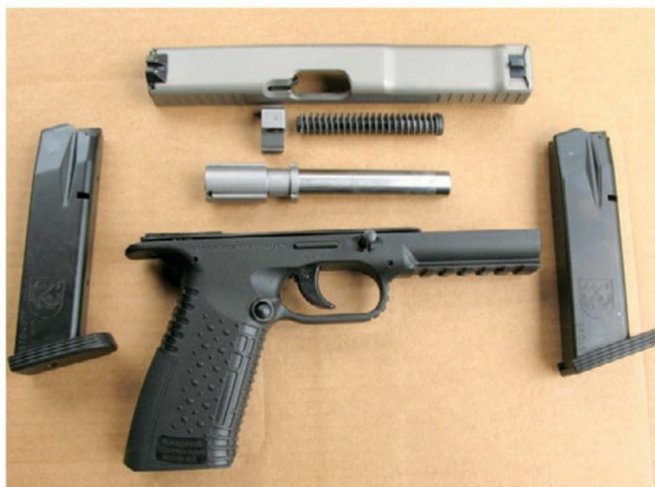
Strike One fieldstripped. Takedown is different but simple. At center is unique locking block that is not attached to frame.
