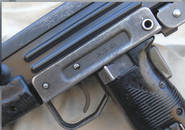
Above: Uzi's grip safety is similar in form and function to that of 1911 pistol, as it must be depressed to retract the bolt or fire the weapon.
