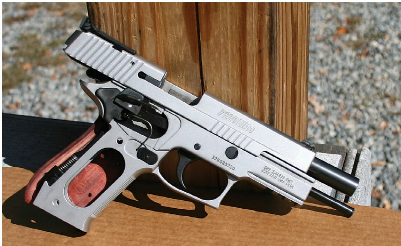
Below: Rosewood grips are wraparound and act as back strap. Hammer's stirrup is enclosed by coil hammer spring. Slide rides on full-length rails.
