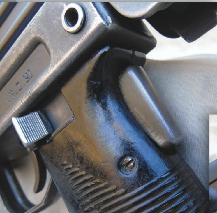
Above: Uzi's grip safety is similar in form and function to that of 1911 pistol, as it must be depressed to retract the bolt or fire the weapon.
