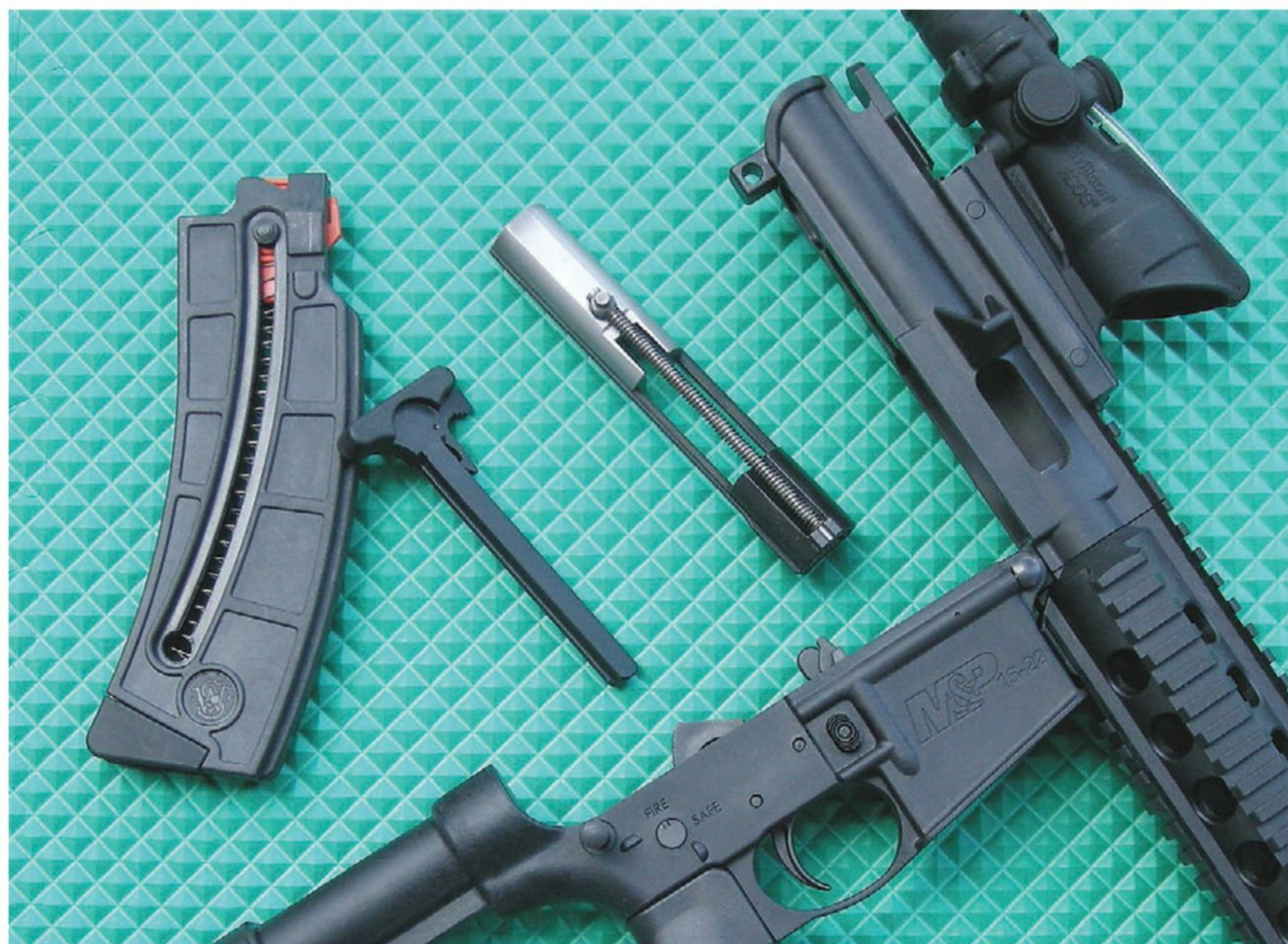
Above: Smith & Wesson M&P15-22 rifle field-stripped with bolt removed for cleaning.
